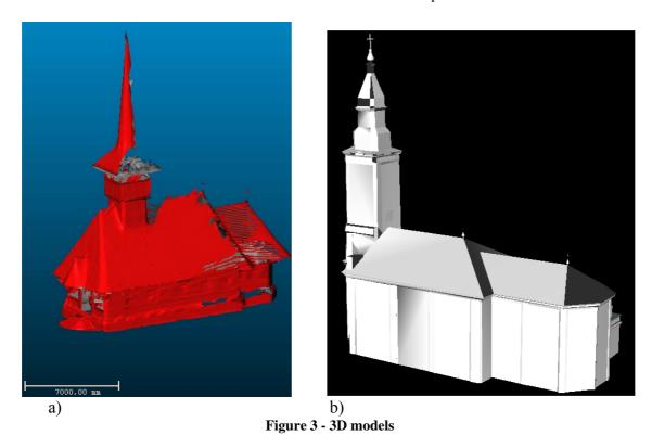
Within this project, for the churches studied it was impossible to use these two methods because of the vegetation and of the buildings which are surrounding the monuments. Therefore the 3D model of the churches was made from the points measured with total station, by using AutoCAD.
